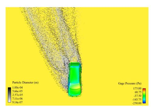
Figure 6: Top view of particle distribution for tire emissions using uniform wind model. Vehicle colored by pressure.
