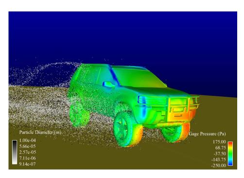
Figure 4: Side view of particle distribution for tire emission using uniform wind model. Vehicle colored by pressure.
