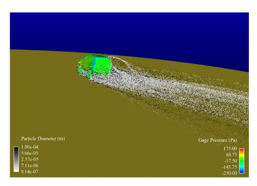
Figure 5: Back view of particle distribution for tire emission using uniform wind model. Vehicle colored by pressure.
