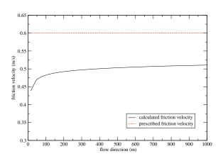
Figure 3: Comparison of prescribed friction velocity and the computed one
