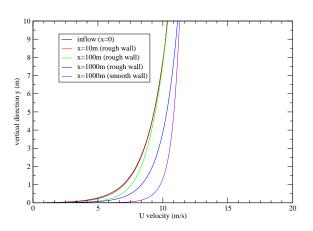
Figure 2: X-component velocity distribution in the vertical direction along the flat plate in the bottom 10m of boundary layer
