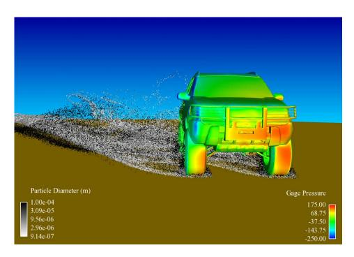
Figure 8: Front view of particle distribution for ground emissions using uniform wind model. Vehicle colored by pressure.
